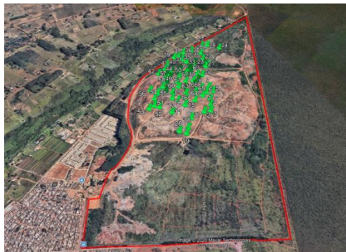
Figure 2. Delimitation of the closed Brasília Jockey Club landfill and spatial distribution of 71 flares.
