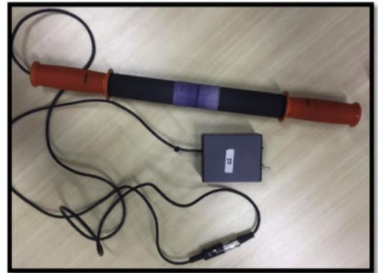
Fig. 2. Roller massage device used. This device was 18 cm in length and 3 cm in diameter with a dense rubberized surface, and it had strain gauges affixed to the roller rod to transmit the signal via Bluetooth to a computer, allowing to control the magnitude of force applied during the intervention.
