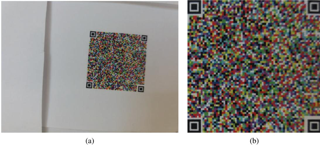
Figure 3.6: HD2DC Version 5, 8-colors, and High error correction level: (a) image snapshot captured at a distance of 7 cm from the camera (Samsung Galaxy J5 ) and (b) rotated and processed version of (a).
