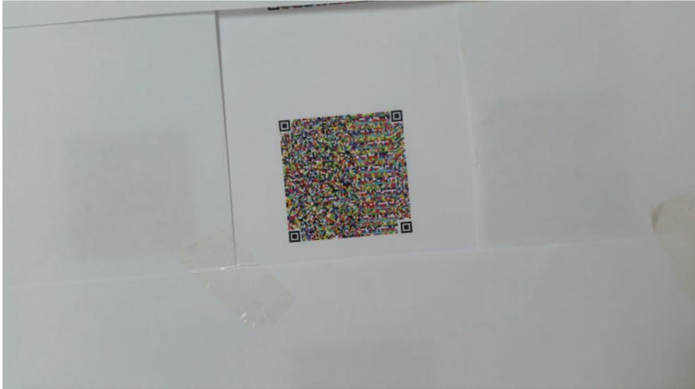
Figure 3.16: HD2DC Version 6 and 8-color, captured and correctly decoded with 5.69% corrupted symbols at a distance of 13cm with the Samsung Galaxy S5 camera.
