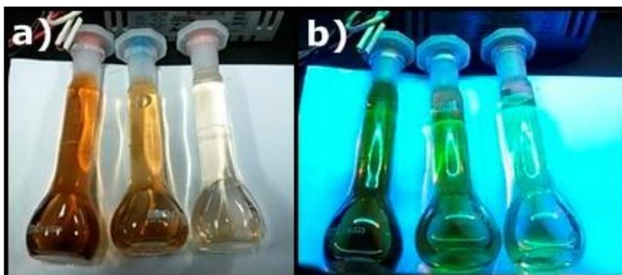
**Figure 6.** Humic substances produced by route I being stimulated by white light and ultraviolet light. (a) HSs under white light. (b) HSs under ultraviolet light with wavelength of 254 nm.
